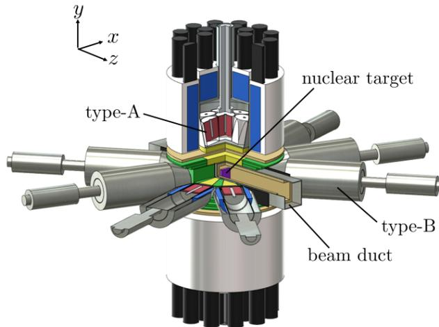
**Fig. 1.** Configuration of the germanium detector assembly in ANNRI.
