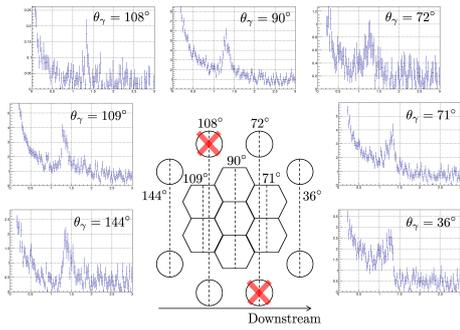
**Fig. 3.** The neutron energy spectrum around the 1.33 eV p-wave resonance, for variable angles accessible at ANNRI. The central figure shows the placement and the shape of each crystal. Two detectors marked by crosses were not available for the experiment (i).
