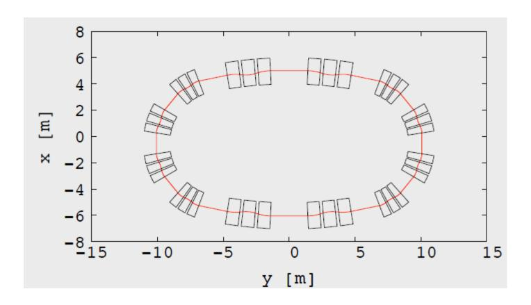
Scaling FFAG with 2 types of circular cells with different k and R matched such that orbit excursion is the same. Again bending is strong in one type contrary to the "straight" section part.
